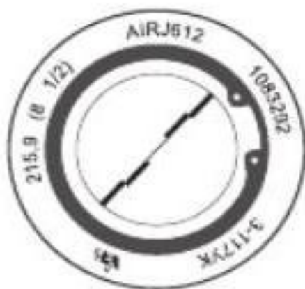
Pin End Face View (Marking)
